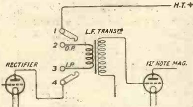
Fig. 2.—Illustrating how the four terminals added to the receiver panel should be connected.
