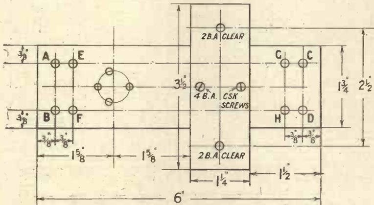
Fig. 3.—Layout and dimensions of the ebonite cross-pieces.
