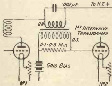
The use of a stabilising resistance across the secondary of the first L.F. transformer may prevent whistling.
