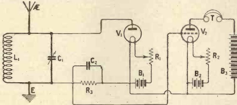
Fig. 3.—Showing a modification of Fig. 2 so that the H.F. component applied to the grid of V2 is eliminated.
