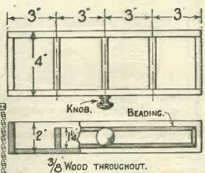
Fig. 3 shows the arrangement of the drawer.
