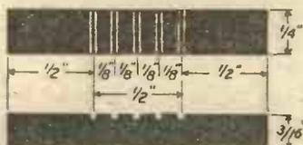
Fig. 4.—Details of the ebonite spacing strips.
