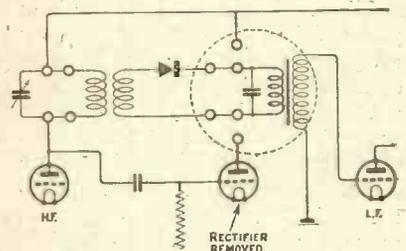
Fig. 6.—The resulting circuit when the crystal is used in place of the valve detector.
