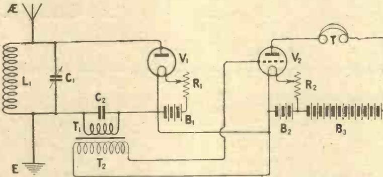
Fig. 6.—A step-up transformer  $T_1 T_2$  has been substituted here for the choke  $Z$  in Fig. 5.
