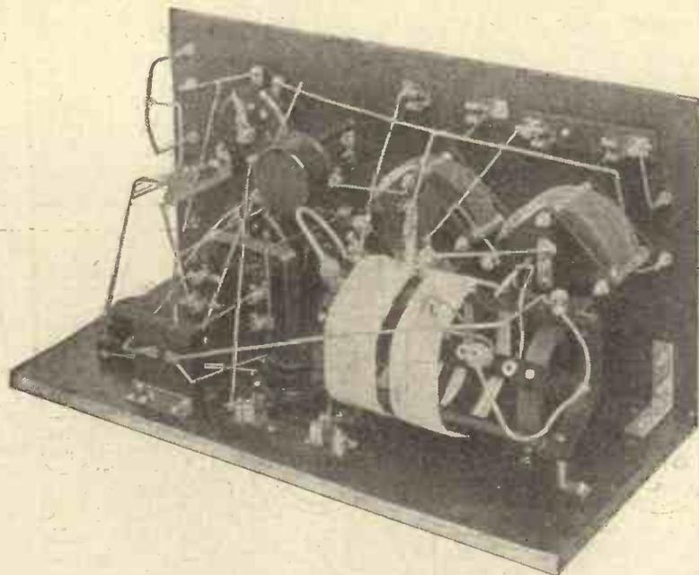
This photograph of the wiring of the receiver also shows the coil with its connections. Note the low-loss former.
