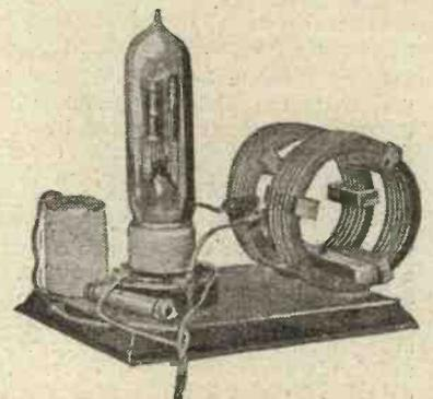
The 20-metre transmitter, including grid and plate inductance, plate choke coil and gridleak.
