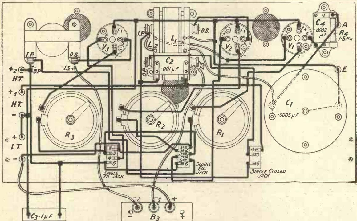
The wiring of the receiver may be followed from this drawing. The connections to the jacks are numbered in accordance with those given in the theoretical circuit diagram. Blueprint No. 102b.
