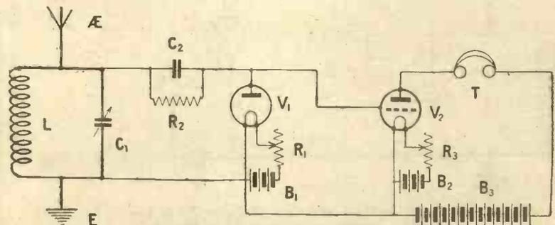
Fig. 2.—In this illustration the detector is a Fleming two-electrode valve followed by a three-electrode valve acting purely as an amplifier and serves to explain the function of the Fig. 1 circuit.
