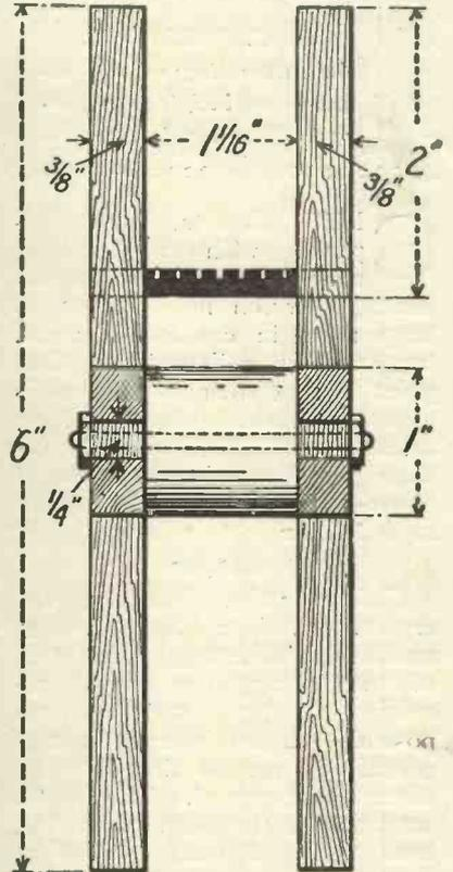
Fig. 5 shows the construction of the coil former.
