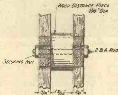
Fig. 3.—The cross-pieces and hub are secured together in a very simple manner.
