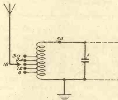
Fig. 2.—The actual connections of the coil.
