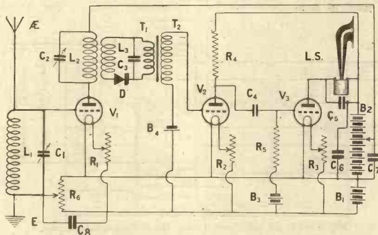
Fig. 1.—In the author's case, the replacing of the valve detector by a crystal results in the circuit shown above.
