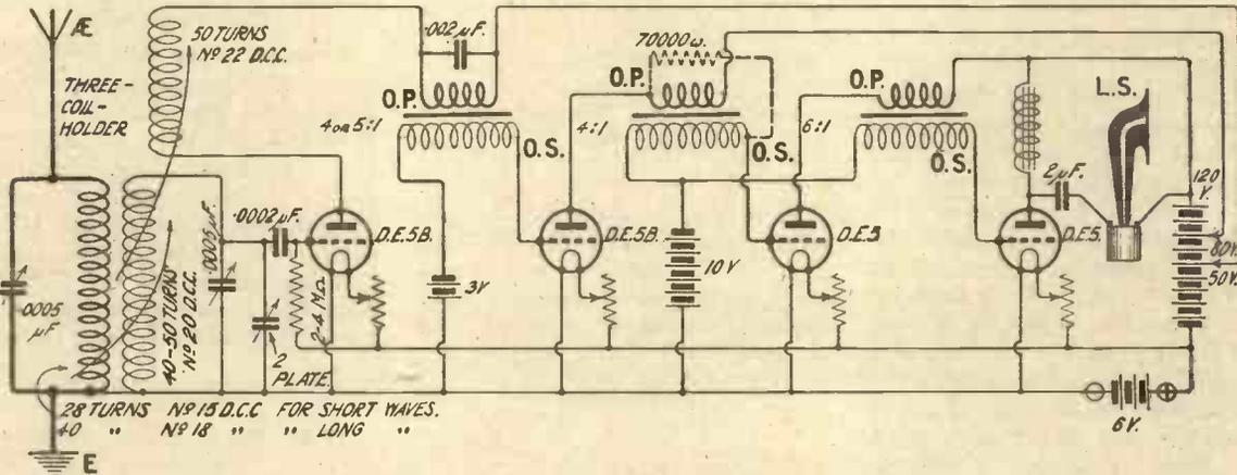
This circuit, in which three stages of transformer-coupled low frequency amplification are employed, gives signals of very commendable quality with great volume. Suitable turn numbers are given for the coils, for covering both the higher and lower sections of the 300-600 metre wave band.
