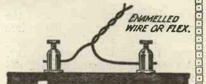
Fig. 4.—The twisted wire method.
