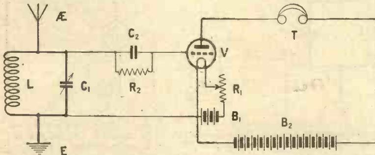
Fig. 1.—A circuit in which the valve V acts as a detector on the leaky-grid condenser principle.
