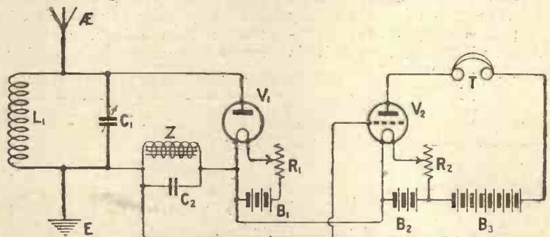
Fig. 5.—The equivalent of the Fig. 4 circuit, two valves being employed in this case to perform the separate functions required. Z, C2 are at the bottom of the anode circuit of V1 for the reasons stated in Fig. 3.
