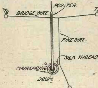
Fig. 3.—Showing principle of the hot wire ammeter.
