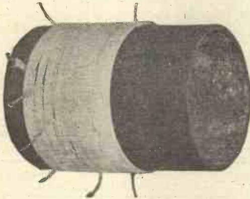
The coil used for the series of simple tests described in this article was of the single layer variety with a number of tapping points.
