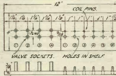
Fig. 2.—Dimensions of the shelf for valves and coils.
