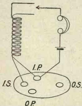
Fig. 2.—How to identify the ends of the windings.
