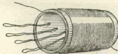
Fig. 3.—By this method the connecting wires are all inside the former.
