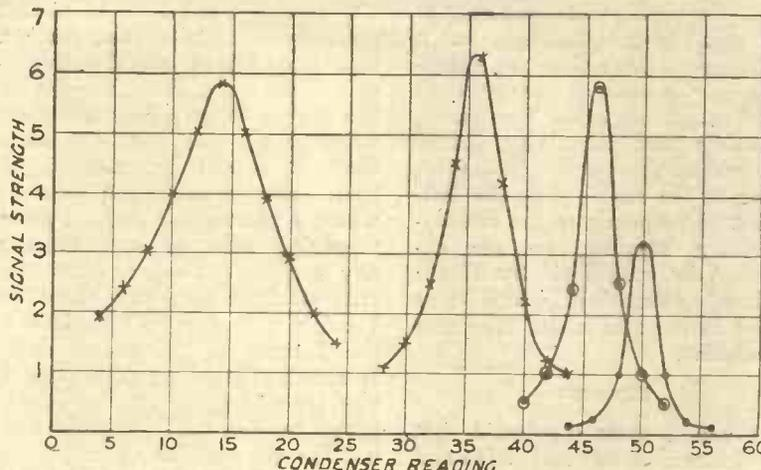
Fig. 3.—These curves express the results obtained by varying the aerial tapping point.
