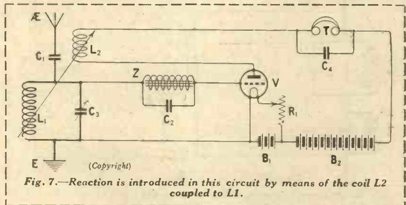
Fig. 7.—Reaction is introduced in this circuit by means of the coil  $L_2$  coupled to  $L_1$ .
