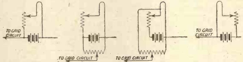
Fig. 9.—Four different connections to the grid circuit which may be tried.
