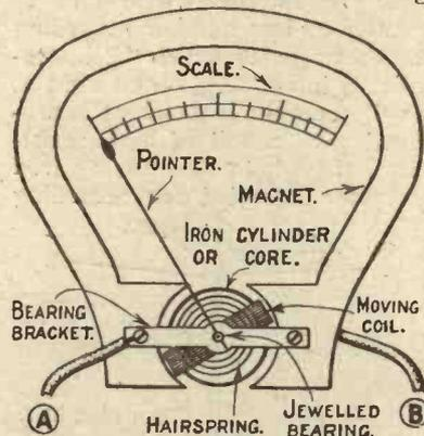
Fig. 1.—Principal working parts of a measuring instrument.
