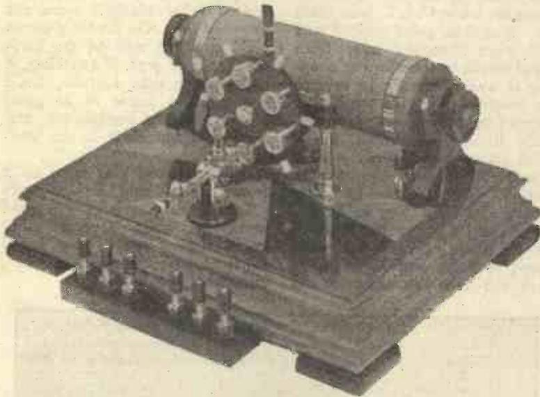
A most handsome crystal receiver made by Mr. T. Orton, a member of the T.O.T. Radio Association of the Underground, before which Mr. Harris recently delivered a lecture. Note the commutator method of tuning on the right hand side.
