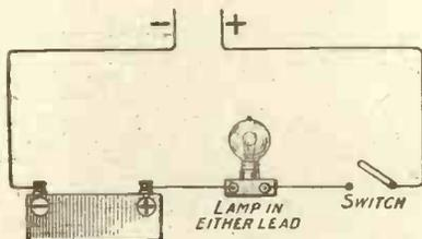
Fig. 6.—How to charge the H.T. accumulator from D.C. mains.
