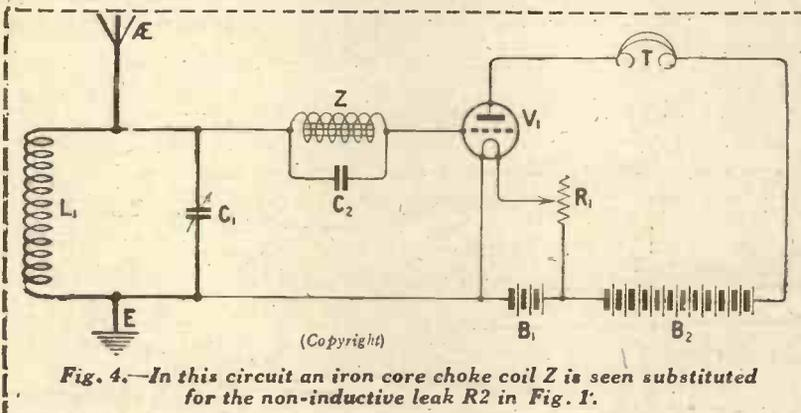
Fig. 4.—In this circuit an iron core choke coil Z is seen substituted for the non-inductive leak R2 in Fig. 1.
