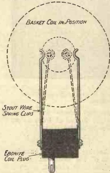
**Fig. 1.—Illustrating the principle.** ebonite coil plug in which the connections are made to screws at the sides, two small pillar terminals, some stout copper wire of No. 16 gauge, and some ebonite,  $\frac{1}{8}$  or  $\frac{3}{16}$  in. thick.
