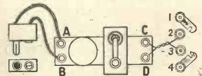
Fig. 5.—The external connections when the unit is used in the set.
