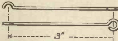
**Fig. 2.—Details of the spring clips.**
