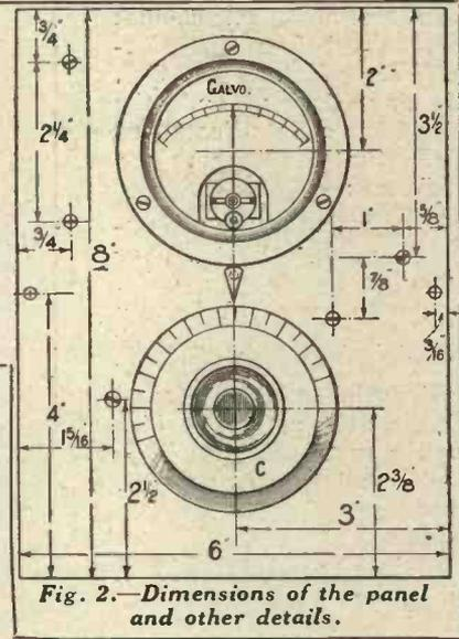
Fig. 2.—Dimensions of the panel and other details.
