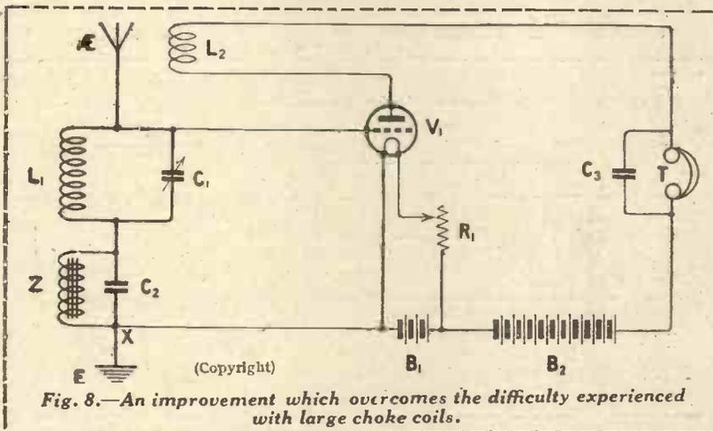
Fig. 8.—An improvement which overcomes the difficulty experienced with large choke coils.
