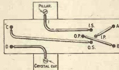
Fig. 4.—How the unit is wired up.
