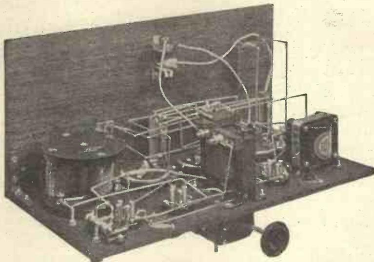
A further view of the wiring showing how the grid connections are made.
