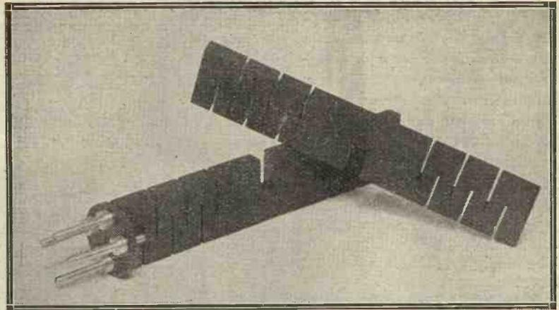
Fig. 5.—The parts of the former ready for assembly.
