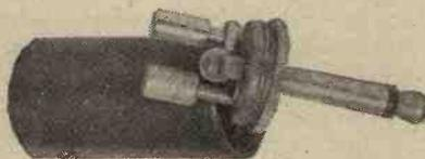
The plug removed from its shield showing how connection is made.
