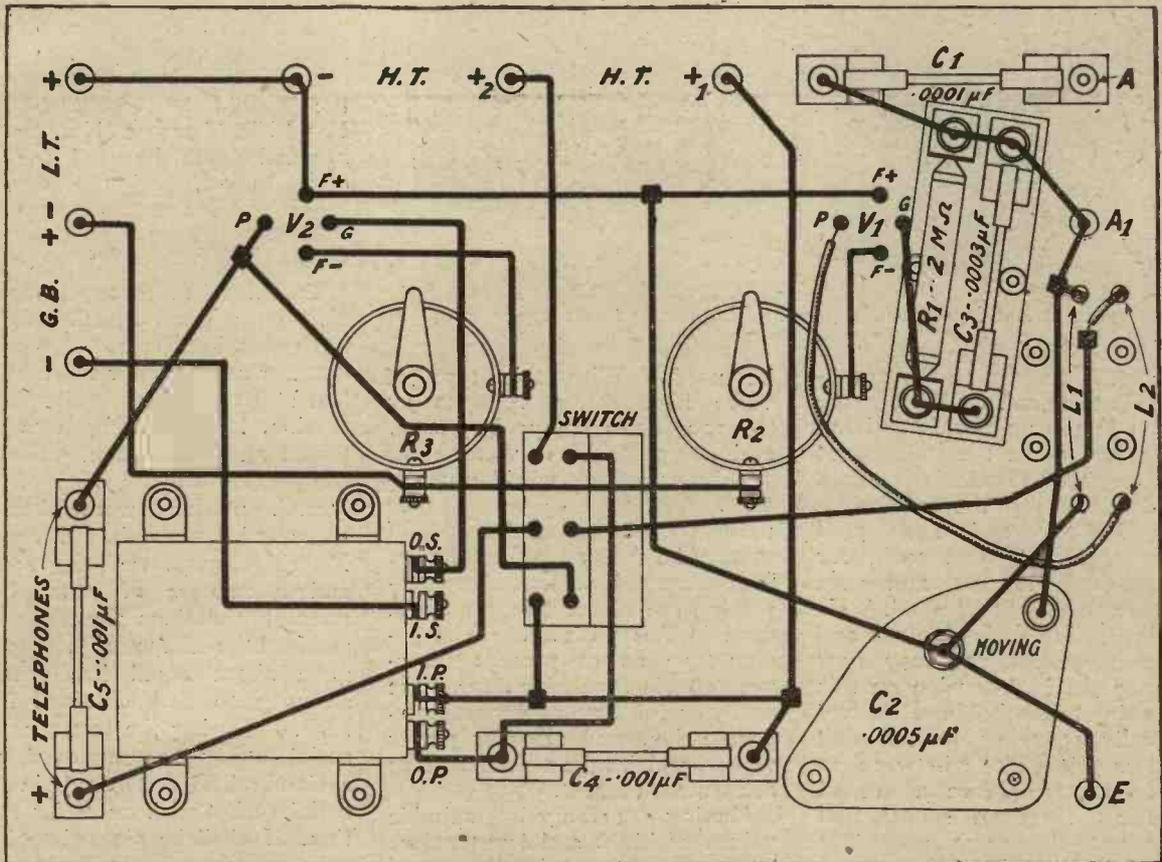
Fig. 4.—The wiring of the receiver may be carried out with the assistance of this practical illustration.
