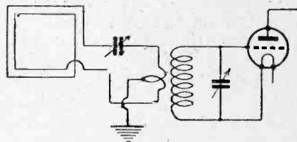
Fig. 5.—In the case of a coupled circuit the middle point of the coupling coil is connected to earth.
