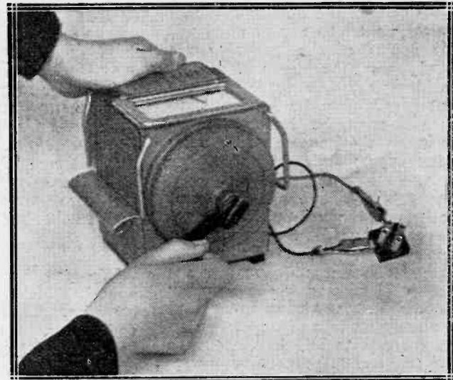
The instrument used by the author in making some of the insulation tests described is of the "Meg" type shown here.
