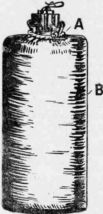
Fig. 3.—Showing how the carbon compound block may be tied up in a piece of cloth.
