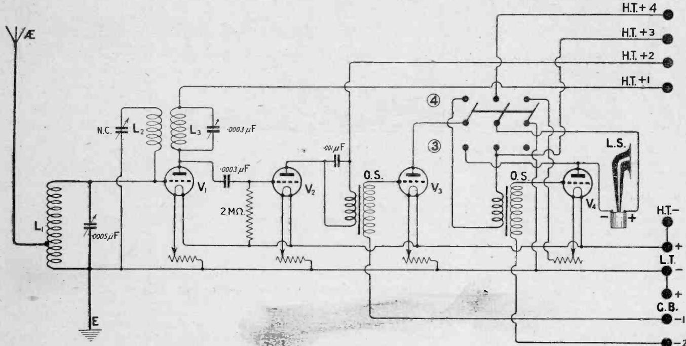
Fig. 1.—The circuit diagram of a selective four-valve receiver, employing a stage of H.F. amplification with neutrodyne control and a switch for providing one or two stages of L.F. amplification. (L. E. S., FOLKESTONE.)
