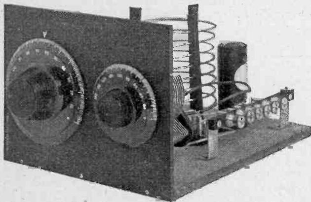
*The two variable condensers are the only components mounted upon the panel of the oscillator.*
