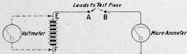
Fig. 1.—Leads from A and B are taken to the component whose leak resistance is to be tested, and a simple calculation from the readings on the meters will then give the value of this resistance.
