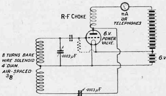
Fig. 2.—The inclusion of a grid condenser and leak, shown dotted in this diagram of the oscillator circuit, may in some cases be an advantage.
