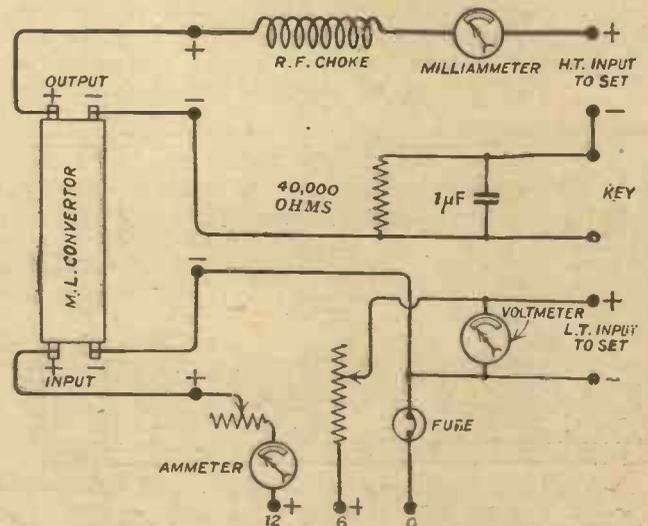
*The negative L.T. and H.T. terminals on the output side are not connected together, and this must therefore be done in the transmitter itself.*
