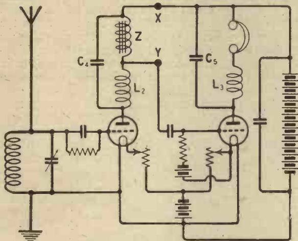
coil Z. This condenser will offer a ready path for the high-frequency currents, and virtually acts as a short circuit for them. Such a condenser will act as a much better conductor for high-frequency currents than for low-frequency.
