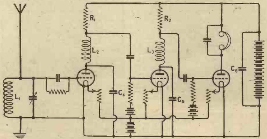
*Fig. 7.—How a resistance amplifier may be compelled to function in a correct manner by means of chokes and by-pass condensers.*
