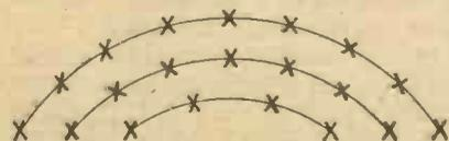
Fig. 3.—Showing how a compass needle can be used to determine the direction of the lines of force at a series of points.
