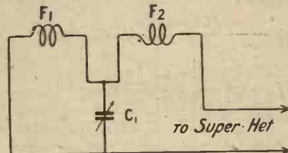
Fig. 2.—In practice the two windings, one tuned and one untuned, are joined in series to obtain the desired neutralisation of the interfering signal.
