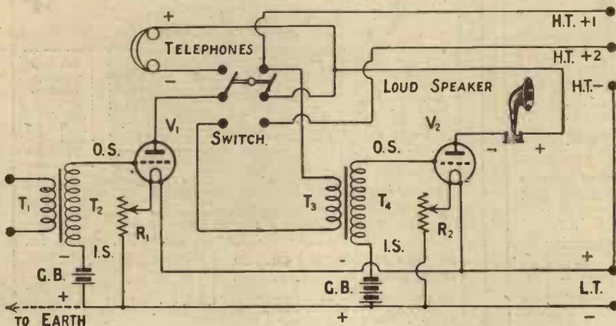
With the switch in the "one valve" position, the filament circuit of the second valve must be broken by means of the rheostat R2.
