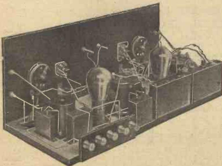
*It is preferable to use separate grid-bias batteries for each stage, while the spacing out of the wiring and components requires considerable attention when a good deal of power is to be handled.*
