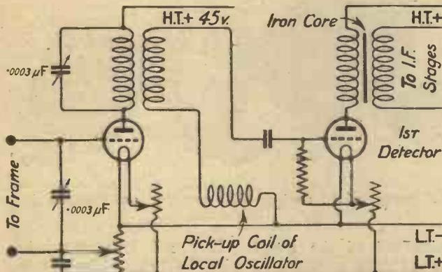
Fig. 1.—The first circuit tried by the author. When used on a frame aerial this proved exceedingly unstable.
