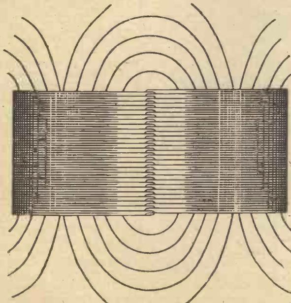
Fig. 6.—The field of the "Bodine" twin-coil transformer was plotted by the compass needle method.
