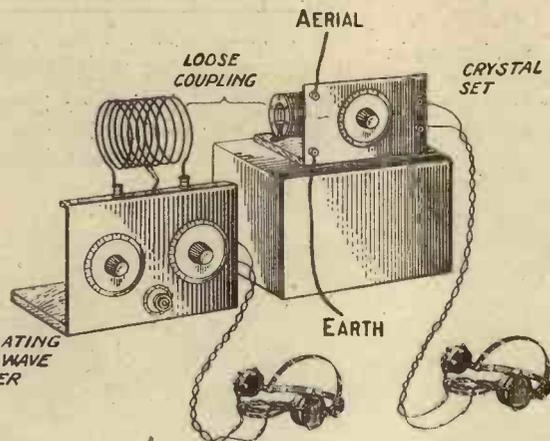
*If the short-wave set is placed beside a crystal receiver strong harmonics of the local station can be picked up with ease.*
