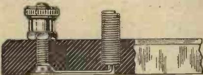
Fig. 1.—A coil of wire wound round a two-inch nail makes good contact with the valve legs.
