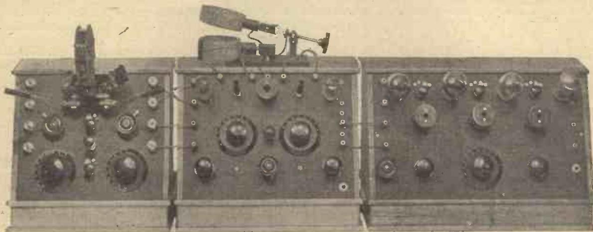
An experimental super-heterodyne which was described by Mr. Kendall in the April 1925 issue of "Modern Wireless." The Tropadyne circuit could be used in this instrument.
