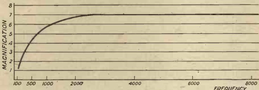
Fig. 4.—Showing the effect of using a choke coupling of unsuitable impedance.
