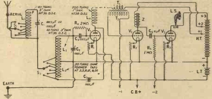
A simplified version of the circuit employed, showing how the switching of the coupling turns of the wave-trap and tuning coils is effected. Note the position in the circuit of the reaction condenser.
