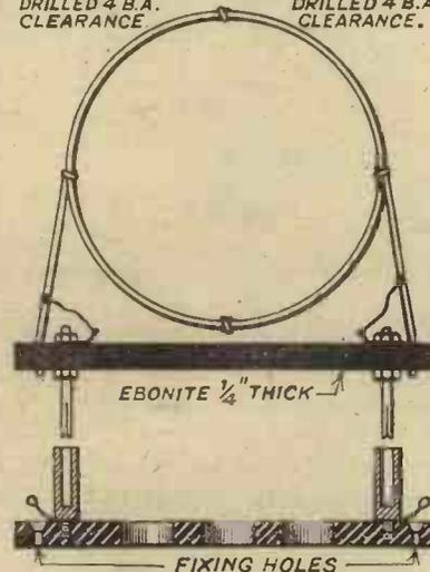
Constructional details of the coils and coil socket.
