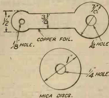
Fig. 1.—The foil and mica are cut to the dimensions shown.
