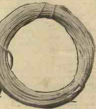
For experimental work any simple home-made coil of adequate size can be used as a choke.
