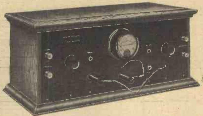
*It is wise in building a power amplifier to include a milliammeter on the panel in order that the correct adjustment of grid bias, etc., may be made most easily by observation of anode current.*
