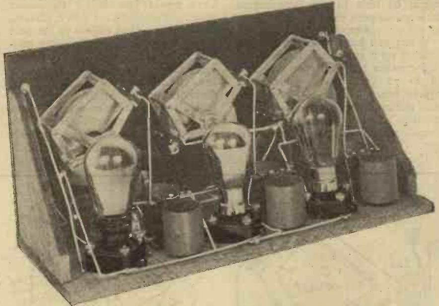
*The set is very compact, yet the coils are well spaced out.*
