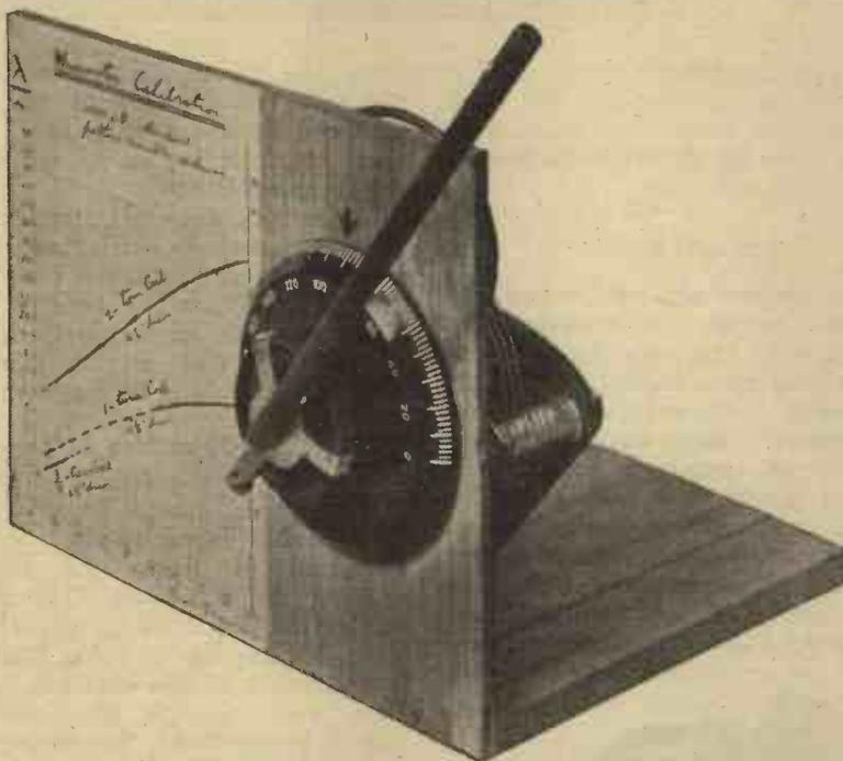
*Extension handles are helpful on the higher frequencies, since it is difficult to eliminate hand-capacity effects by any other simple method.*
