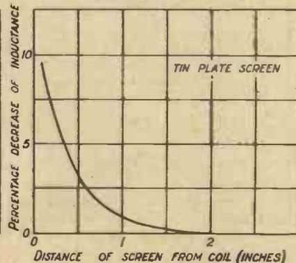
Figs. 8 and 9.—The screening effect depends on the shape of the coil, and is smaller with a long coil than with a short one. Compare these curves with those in Figs. 2 and 3.
