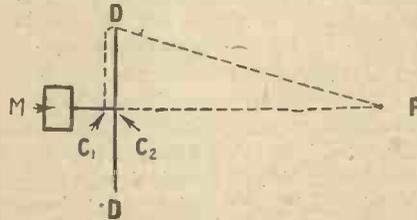
Fig. 12.—A listener at the point P may hear sounds from both sides of the diaphragm D, as indicated by the two dotted sound-paths C<sub>1</sub>-P and C<sub>2</sub>-P.
