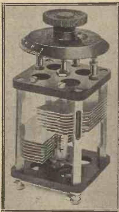
Dielectric material is sometimes "economised" in the electrical sense by drilling large holes in the end plates.
