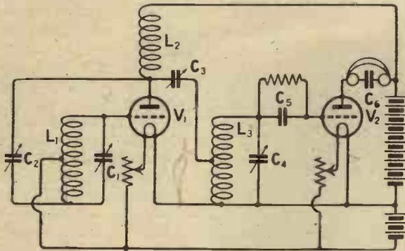
Fig. 5.—This circuit, although capable of being stabilised, only applies half of the available voltage to the grid of V1.
