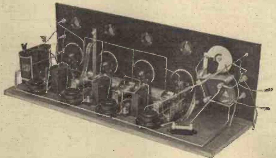
The design of a set with three resistance stages calls for some care in lay-out.
