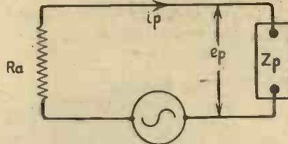
Fig. 2.—In this diagram the valve is represented as a source of alternating voltages.
