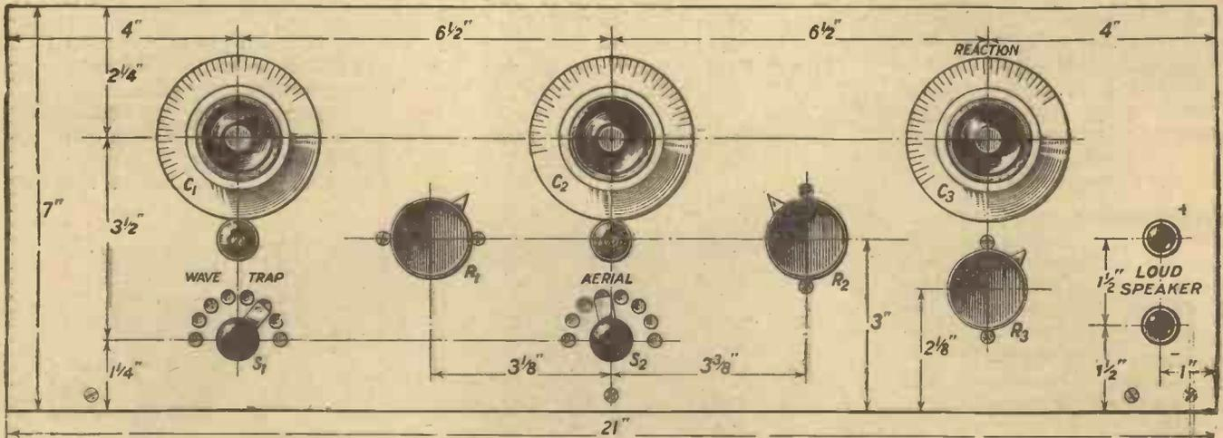
In making an exact copy of the original set this drilling diagram should be used. The only terminals on the front of the set are for the loud-speaker, those for aerial and earth and batteries being placed on strips attached to the rear edge of the base-board.
