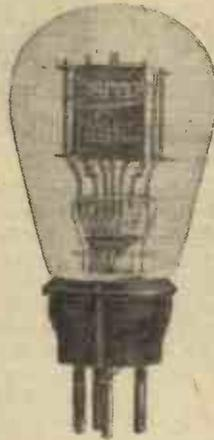
The latest type of D.E.4 valve has a pipless bulb.
