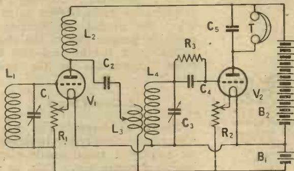
Fig. 3.—In this circuit a shunt coupling scheme is employed.
