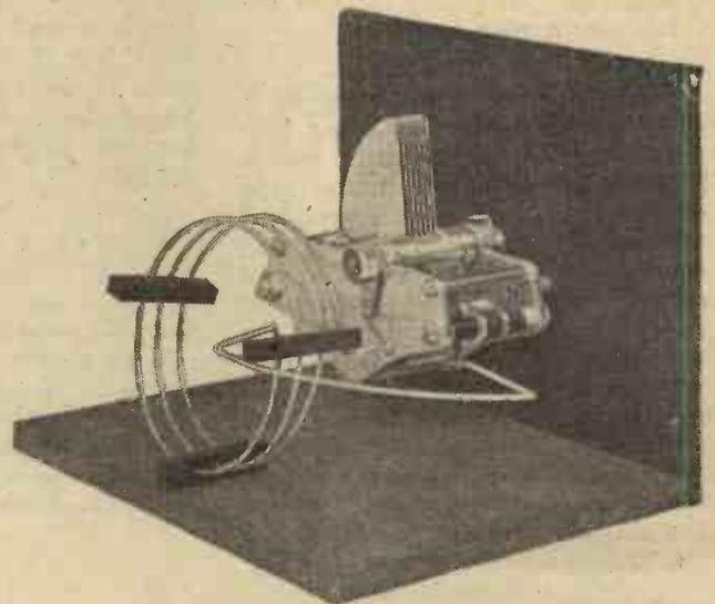
oscillating over a wide band, loosen it. The ideal position is that in which little more than a single click is heard. Note this position, and obtain as many more of these calibration points as possible, plotting frequency (or wavelength) against scale readings in the usual manner.
