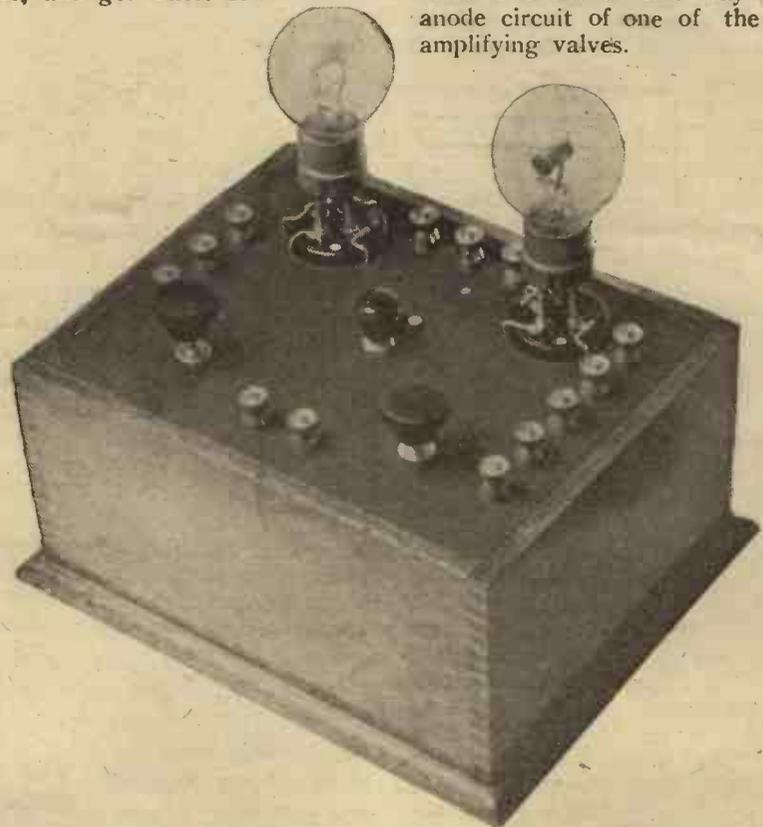
For experiments with resistance amplifiers a very simple instrument is to be preferred.
