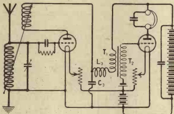
both high- and low-frequency currents are passing through this resistance, potentials will be set up across the battery and may cause obscure reaction and other interference effects. These may be cut out by the short-circuiting process of using a condenser in parallel with the battery.
