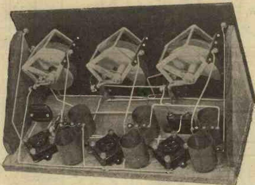
*This view with the valves removed shows clearly how the parts are laid out on the base-board.*
