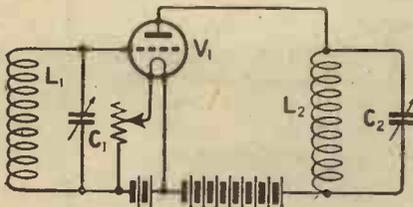
Fig. 6.—This skeleton circuit shows that the internal impedance of the valve may be considered as being in parallel with the tuned circuit L2C2.
