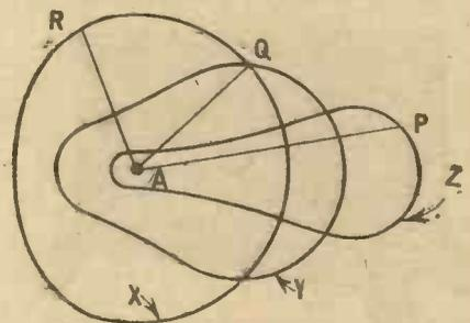
Fig. 11.—The outlines X, Y and Z represent the relative distributions of three different frequencies from the loud-speaker at A.
