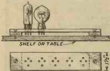
The construction of the rack.
