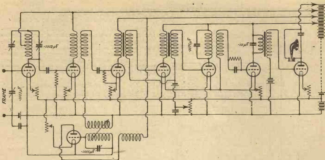
Fig. 5.—The most successful arrangement tried. Two stages of H.F. precede the first detector.
