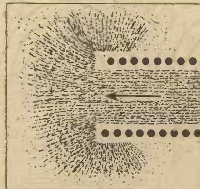
Fig. 4.—Iron filings arrange themselves in this way in the field of a solenoid coil.
