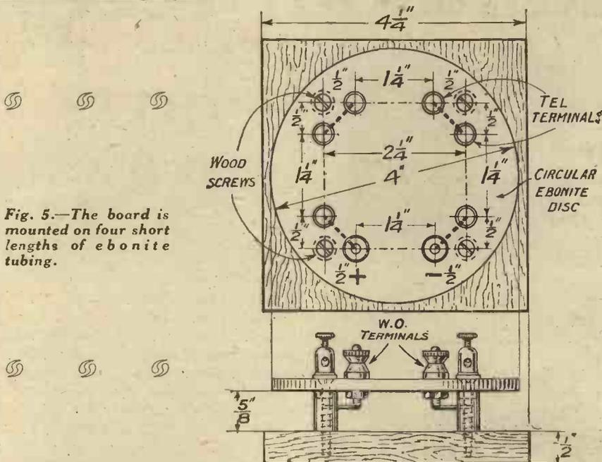
Fig. 5.—The board is mounted on four short lengths of ebonite tubing.
