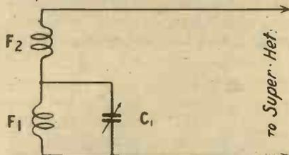
Fig. 3.—These are the connections of the split-winding frame aerial illustrated on this page.
