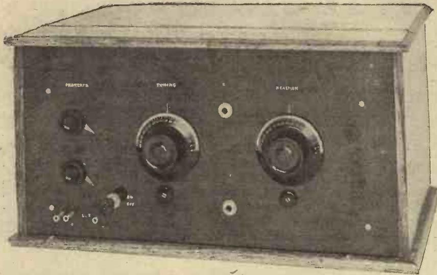
The tuning controls are placed in positions which make for ease of operation; the rheostats are mounted on the left to simplify the wiring.
