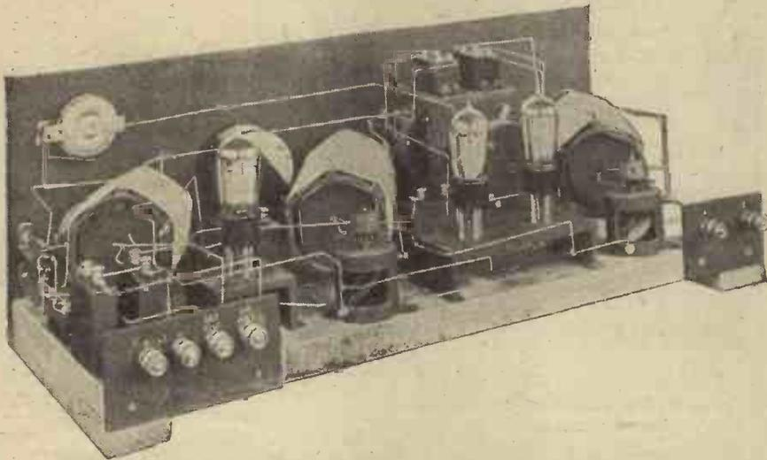
The battery and aerial and earth terminals are placed on ebonite strips at the rear of the baseboard.
