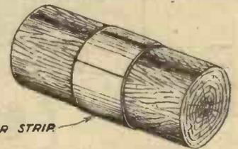
Fig. 3.—The paper strip is wrapped round the wooden cylinder as shown.
