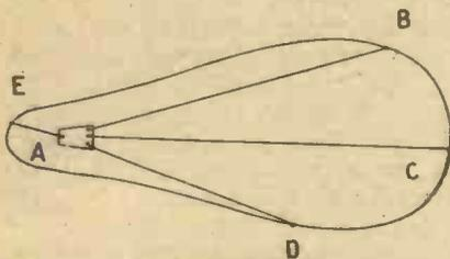
Fig. 10.—Illustrating the distribution of a single frequency from a horned loud-speaker situated at A.
