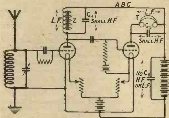
Fig. 3.—The condenser C4 helps to reduce the parasitic H.F. troubles.
