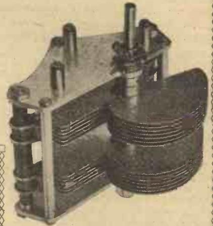
*One of the more recent types of "low-loss" condenser (Igranite dual) in which the fixed plates are supported by side pillars of insulating material.*
