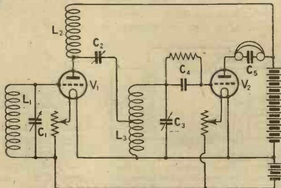
Fig. 4.—By making C<sub>2</sub> variable a fixed connection to L<sub>3</sub> may be employed (compare with Fig. 3).
