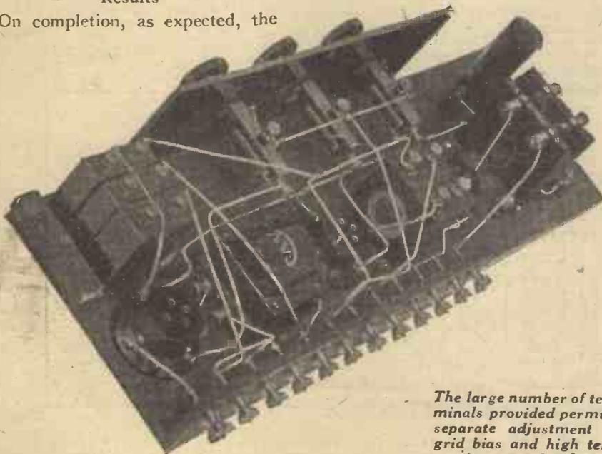
The large number of terminals provided permits separate adjustment of grid bias and high tension on each valve.
