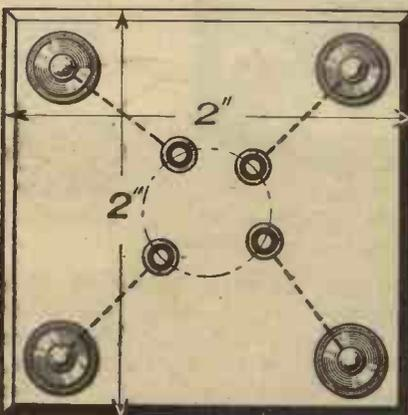
Fig. 2.—The drilling diagram for the valve-holder.
