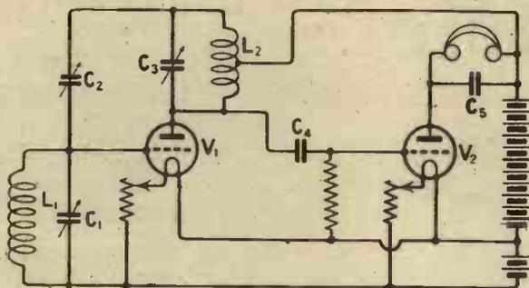
Fig. 7.—This circuit yields improved selectivity as a result of the splitting of the coil L<sub>2</sub>.
