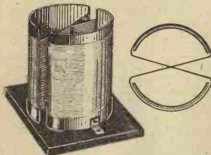
The "D" coil, an example of the astatic or non-pick-up type.
