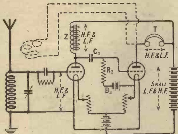
*Fig. 1.—If the reaction coil shown by dotted lines is inserted it can be shown that considerable H.F. currents are flowing in the anode circuit of the second valve.*
