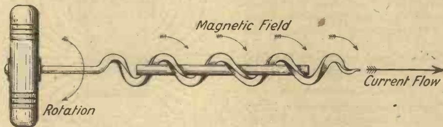
Fig. 2.—A useful rule for the direction of a magnetic field can be memorised with the aid of this diagram.
