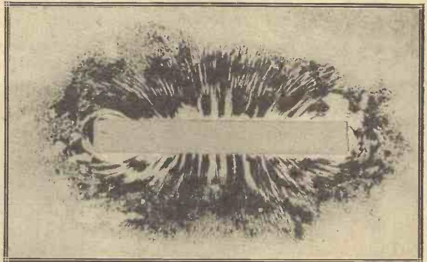
A photograph of a coil field as indicated by the iron filings method. This was "coil A."
