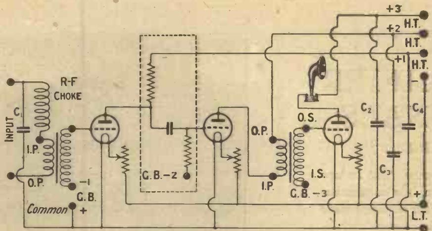
Fig. 1.—The circuit incorporates two stages of transformer coupling and one of resistance-capacity.
