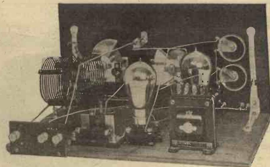
The high-tension positive and aerial connections are made to a strip at the rear of the set. The position of the coils is clearly visible.
