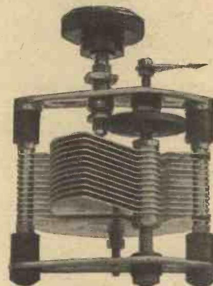
Another method of supporting the fixed plates with a minimum amount of dielectric material is illustrated here.
