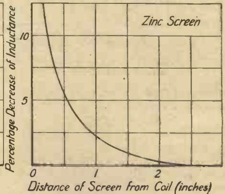
Figs. 6 and 7—The use of zinc for the screen gives results similar to those for copper. If the screen is not nearer than two inches the effect is practically negligible.
