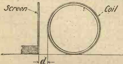
Fig. 11.—In the final experiments the effect of placing the screen at the side of the coil was investigated.
