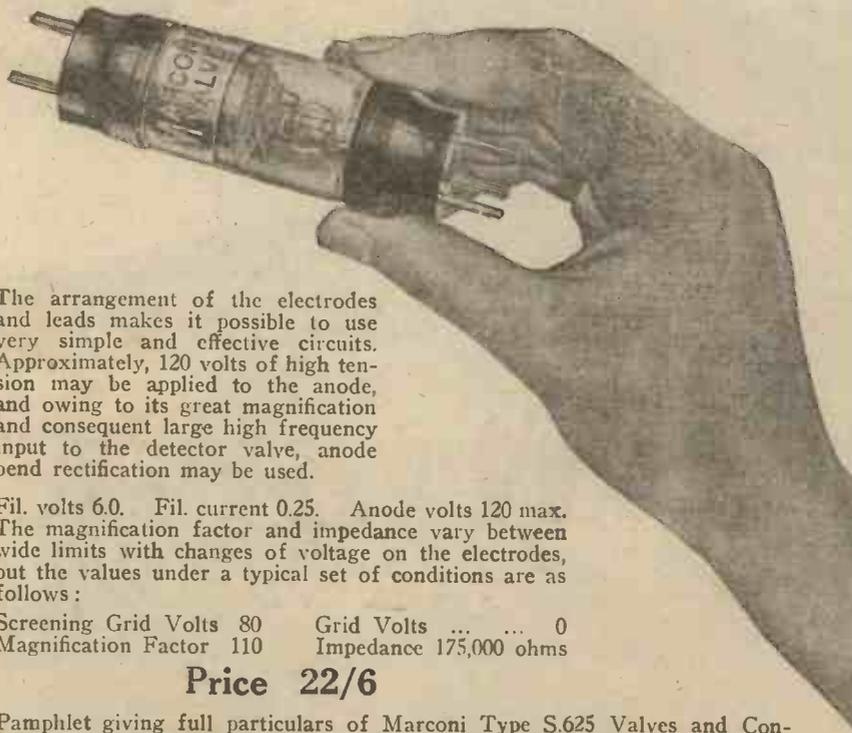
The arrangement of the electrodes and leads makes it possible to use very simple and effective circuits. Approximately, 120 volts of high tension may be applied to the anode, and owing to its great magnification and consequent large high frequency input to the detector valve, anode bend rectification may be used.
